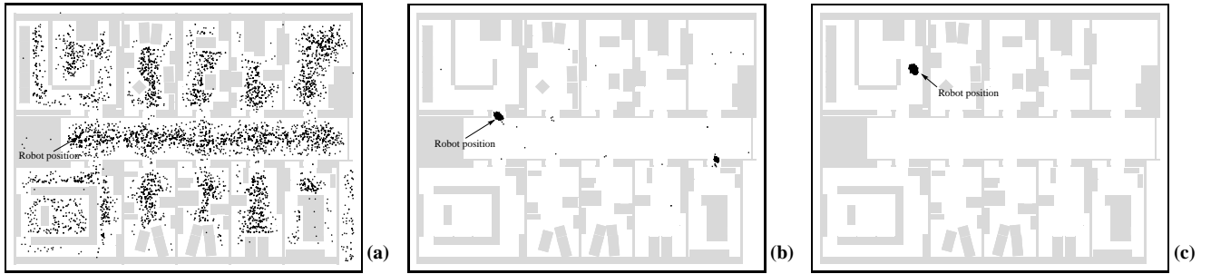
Fig. 4: Global localization: (a) Initialization, (b) ambiguity due to symmetry, and (c) achieved localization.
