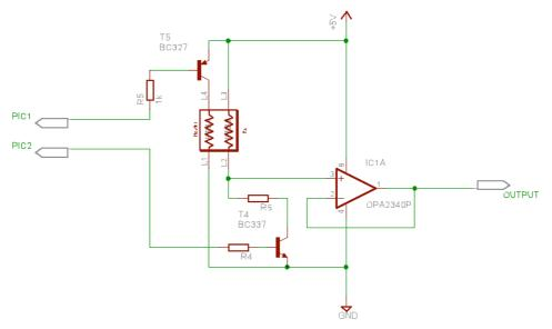
Fig. 33: Carbon Monoxide Sensing Circuit
