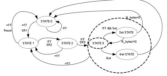
Fig. 45: Motor State Machine
