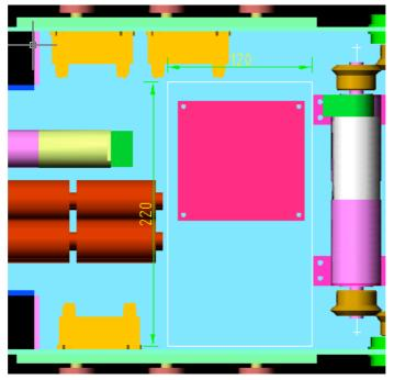
Fig. 22: Available space for the PC and remaining electronics
