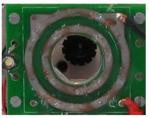
Fig. 57: Concentrical voltage connectors
