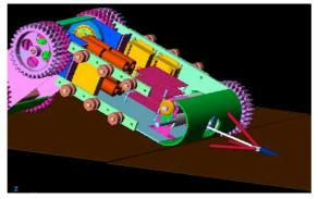
Fig. 24: Robot lowering its back to facilitate docking
