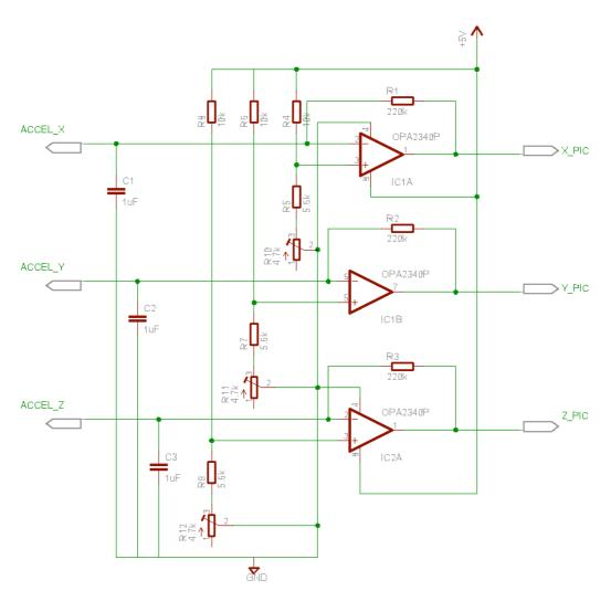
Fig. 35: Accelerometer Adaptation Sub-Circuit
