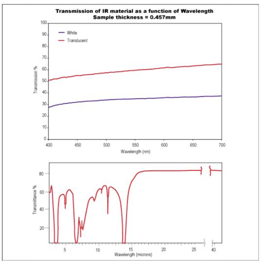
Fig. 59: Transmission of IR plastic
