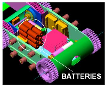
Fig. 21: Localization of the battery packs
