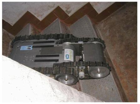
Fig. 66: Robot going downwards through stairs
