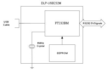
Fig. 28: DLP-USB232M USB to RS232 Bridge
