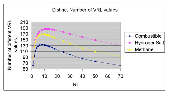
Fig. 71: Number of distinct samples at 8 bits versus Load Resistance
