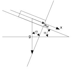
Fig. 3: Finding the inclination angle  $\alpha$  by measuring static acceleration
