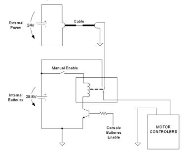
Fig. 37: Motors Power Supply
