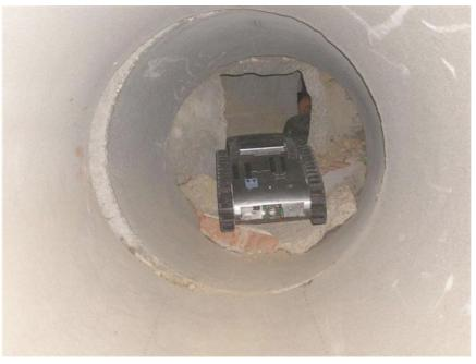
Fig. 65: Robot going through a wrecked pipe to find a person
