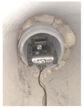
Fig. 69: Raposa on Empty water pipe
