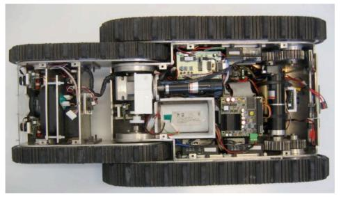
Fig. 46: Robot Inside View
