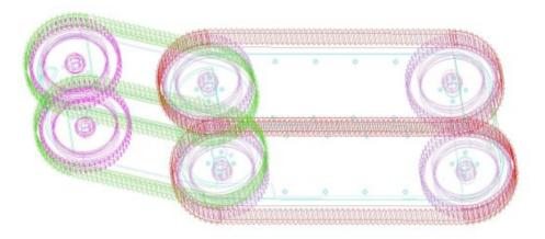
Fig. 16: The main body and arm tracked wheels
