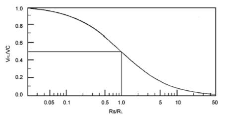
Fig. 70: Resolution versus Load Resistance
