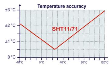
Fig. 43: Temperature Accuracy
