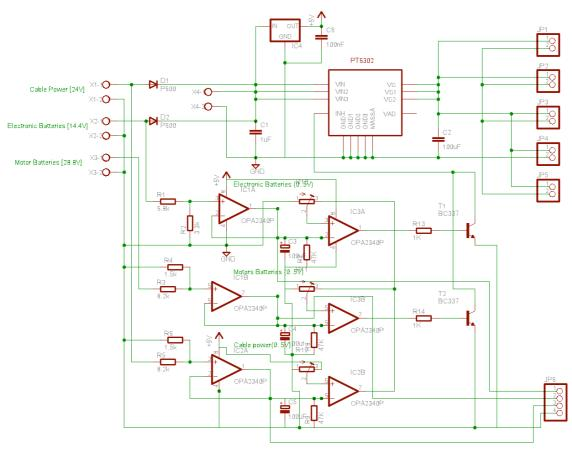
Fig. 38: DC-DC and voltage monitoring electrical circuit
