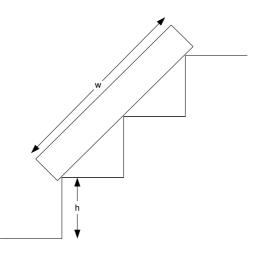
Bad: The robot only has one stand point. It looses its current inclination, making impossible to climb the next step. Good: The robot has at least two points where to stand on and keeps its orientation. So, it grabs the next edge in a more favourable way.
