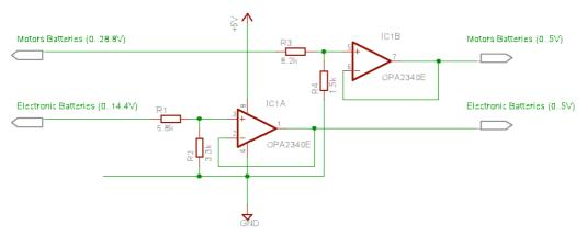
Fig. 39: Voltage Monitoring
