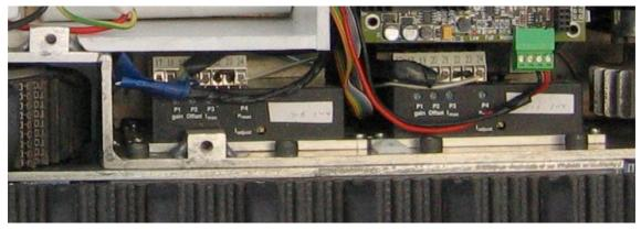
Fig. 49: Controllers attached to the aluminum plate
