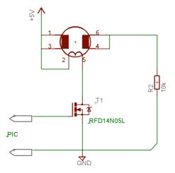
Fig. 31: Generic Gas Sensor Circuit
