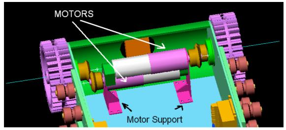
Fig. 18: Locomotion Motors and its support structure
