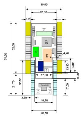
Fig. 17: Robot top view and dimensions in cm.
