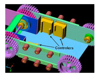
Fig. 20: Motor controllers
