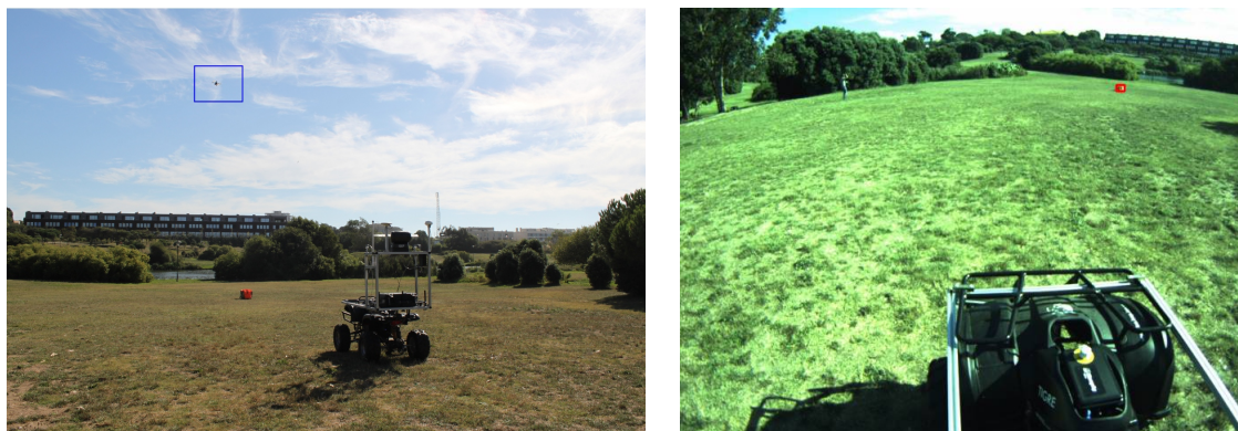
Figure 4.12: Left: Orange static target being tracked by both vehicles: the (UGV) TIGRE and (MAV) Pelican, as shown in the blue box. Right: field of view of TIGRE's left camera tracking the orange static target assembled with a (RTK) (GPS) Ground Truth System.
