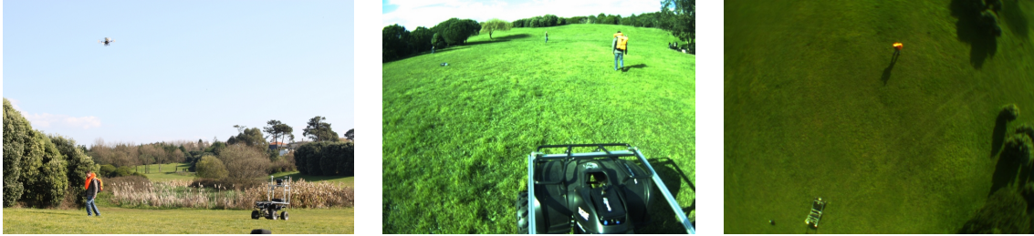
Figure 4.22: Dynamic target tracking experimental case. Left: Orange life jacket being tracked and followed by both vehicles. Middle: Field of view of the UGV TIGRE's left camera tracking the dynamic target. Right: Field of view of the (MAV) PELICAN's downward camera.
