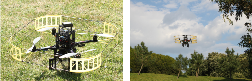
Figure 4.9: Asctec Pelican Micro Aerial Vehicle
